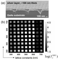
Fig. 1. (a) SEM image of a plasmonic crystal in cross section. (b) SHG image of an array of plasmonic crystals of various lattice constants, showing the effect of plasmonic band gap at periodicity 650 nm. The intensity scale is logarithmic.
