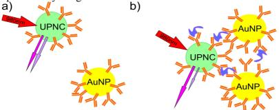
Fig. 1. Functional diagram of the biosensor. a) state in the absence of protein, b) state in the presence of protein. Emission of UPNC is modified by the plasmonic effect of AuNP.
