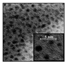
Fig. 1. TEM images of AuAgGSH nanoparticles.
