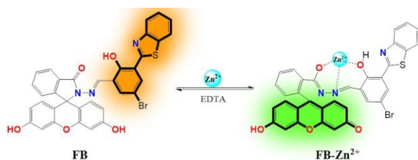
Fig. 1. The proposed mechanism for Zn^{2+} detection by FB
